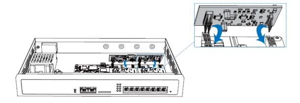
**STEP 3** Insert a SIM card on the GSM/3G module following the instructions. Skip this step if no GSM/3G module installed.
